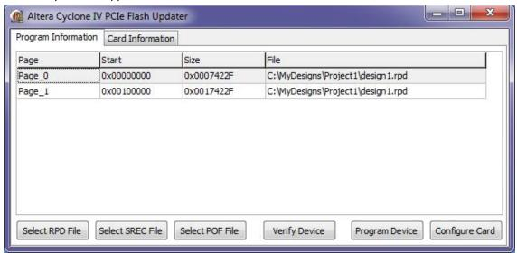
If the update fails then the device will failsafe and the card will still appear as an "Altera Cyclone IV PCIe EPCS update device".
