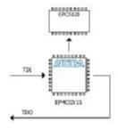
In Altera's remote update solution there are two or more configuration images. A factory default logic design and one or more user logic designs. The factory default logic and the user logic are completely independent of each other and reside in different parts of the EPCS flash. The factory default image is at the start of the EPCS flash and the user logic is at different, known, offsets.
