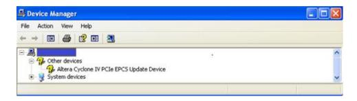
MEV provide a Windows application that talks to the "Altera Cyclone IV PCIe EPCS update device" and allows the user image to be updated in EPCS flash. There is an SDK for this interface too so you can write your own applications.
