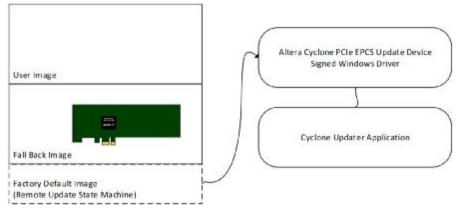
To use the Altera Remote update solution both the factory default design and the user designs need to include a special dedicated hardware IP block provided by Altera called the Remote Update IP. They also need to be built in remote configuration mode. This allows the designs to access the embedded FPGA features that are designed to facilitate remote update.
